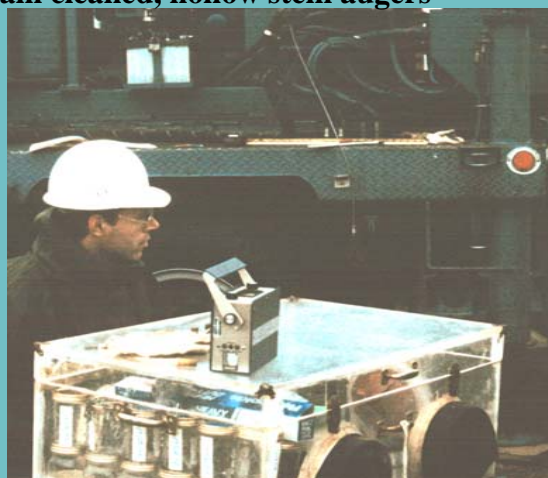
Core barrels extruded in nitrogen filled glove box, into 20 mL soil microcosm vials using sterilized, disposal syringe barrels
